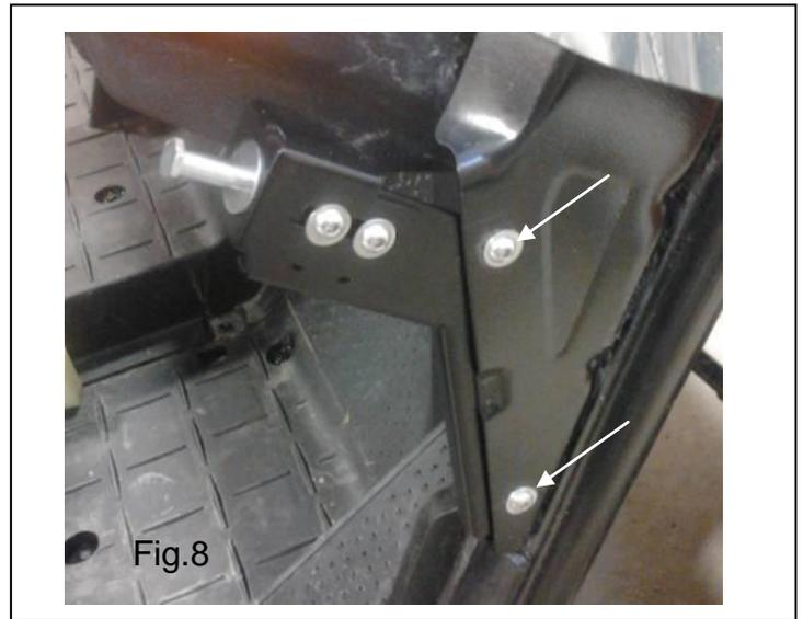
**Tip:** It is easier if you put together the parts required as shown here (Fig.8-2) before fastening to the bike. The main bracket (A) is attached to the adjustment bracket (B) using (2) ¼-20 x 0.75”L screws, washers & nuts. The striker bolt (C) can then be fasten using the 5/16-18 nut (D).
