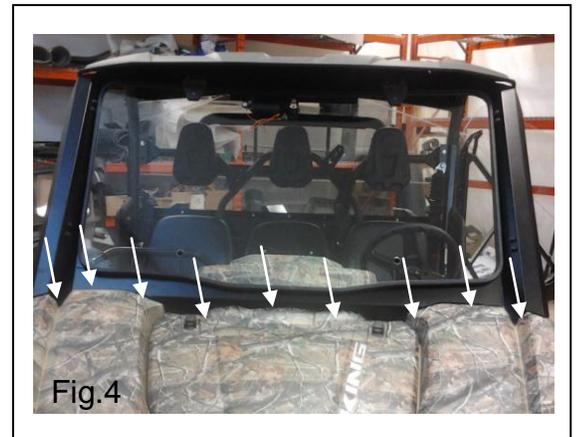
**v)** Adhere low density foam gasket to top portion of hood using marker line as centerline guide to ensure windshield panel will sit squarely onto foam after installation.
