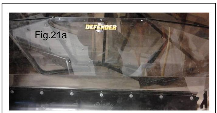
**xx)** With dump box open, re-install rear panel with (4) ¼"-20 x 0.5"L hex screw & seal washers as shown. Fasten the top of the panel to the roof using (2) ¼"-20 x 0.5"L hex screw & seal washers as well.
